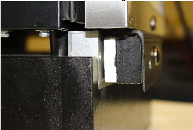
Close up of magnet and armature with door closed
